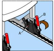
Close handles B to lock the chair in its new position. The safety bolts A should rest in their lower position
