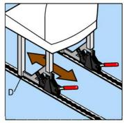
By gently tilting the seat forward onto the plastic pads D at the front of the seat, slide the seat back and forth to your preferred position\*
