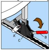
While holding safety bolt A in its upper position pull handles B away from the Millennium 2 fitting C to unlock.
