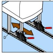
By gently tilting the seat forward onto the plastic pads D at the front of the seat, slide the seat back and forth to your preferred position. Legs with front Spigot must sit in the track hole in your preferred position
