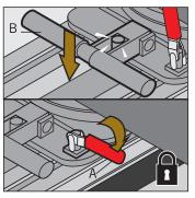
Let go of handle B and it will automatically drop into the next available hole as you slide the base. Then push down the red toggle A until it can't move to lock the base.
